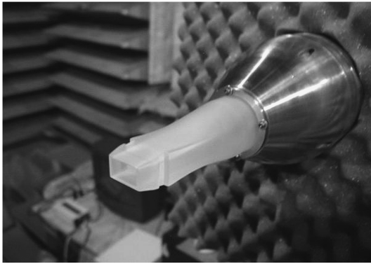
Fig. 1 Rectangular stereo lithography nozzle attached to plenum inside the anechoic chamber of the high-speed jet noise facility.
